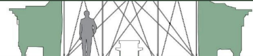
Prof. Eng. Lorenzo Jurina and Eng. Edoardo Radaelli, creators of this unprecedented consolidation, define it as a parabolic hyperboloid (HYPAR), a sort of "hourglass" system that, in the event of an earthquake, will be able to counterbalance the compression of the masonry on both sides of the tower.
