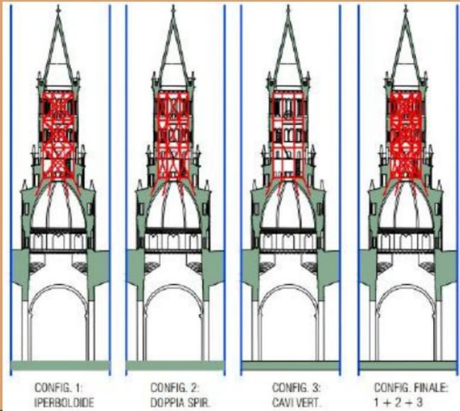
**2.** To ensure resistance to bending and torsion, some cables will be arranged according to a "double spiral" geometry such as to form vertical "X", parallel and adjacent to the frame of the masonry.
