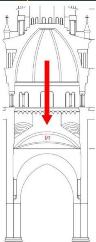
The high mass of the tower, to which is added that of the heavy cusp at its top, has led over time to the formation of cracks and subsidence in the area of the triumphal arch and in the vaults of the presbytery and the north transept.
